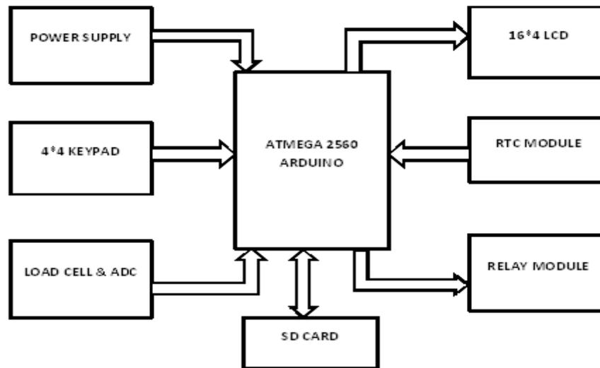
Fig. Block diagram of the system
